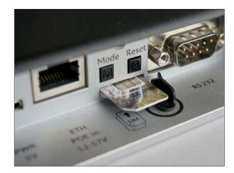
Position SIM card lock into position as indicated on a photo. Gently insert SIM card into upper slot.
