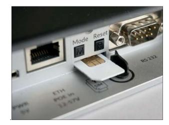
Positilon SIM card lock into position as indicated on a photo. Gently insert SIM card into lower slot.
