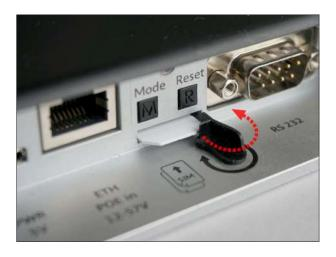
Rotate SIM card lock into position as indicated on above photo to lock SIM card.
